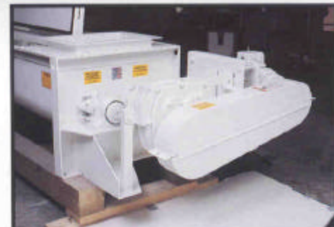
Shaft mount drive with torque flex belt drive
