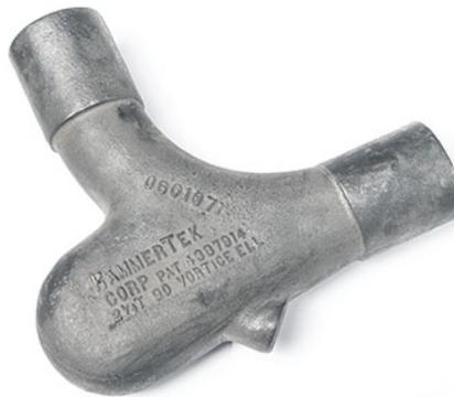
*The deflection elbow's short radius, vortex design features a protruding spherical chamber that causes a ball of material suspended in air to rotate, gently deflecting incoming material around the bend without impacting the elbow wall or generating heat.*
