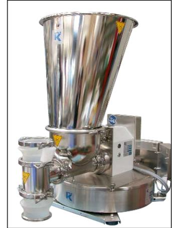
KTron LIW Pharma feeder on a D5 scale
