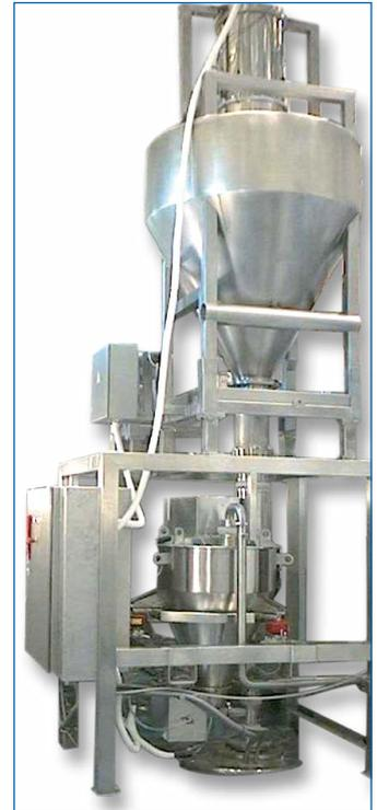
K-Tron P-Series pneumatic receiver and LIW feeder with IBC dispensary station
