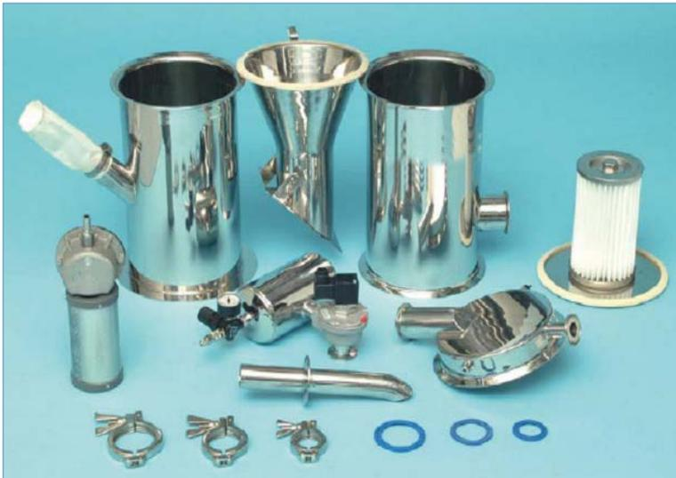
P Series vacuum receiver disassembled for cleaning
