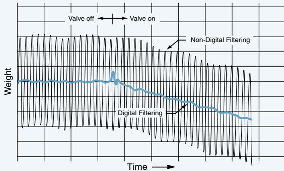
*In vibration-prone environments digital filtering permits accurate detection of even small variations in weight, where conventional filtering techniques fail to discriminate between the forces induced by vibration and actual weight changes.*
