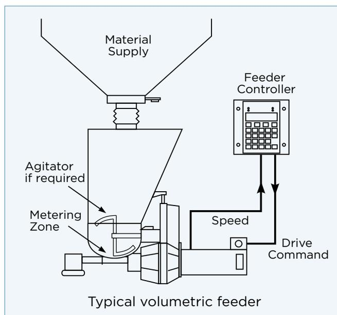
drastically and unpredictably. For sticky materials, buildup on the screw lowers the volume-per-revolution relationship, throwing off calibration. Floodable powders, when aerated, can flow uncontrolled through the screw, rendering volume per revolution meaningless. And friable or other materials whose density can vary greatly limit the potential for high accuracy when fed on a volumetric screw feeder.
