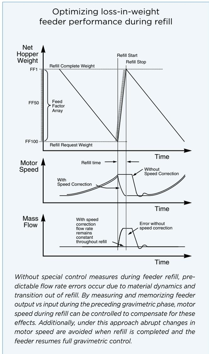
made to this array of feed factors, and the appropriate motor speed can be applied based on sensed system weight as the hopper is filled.
