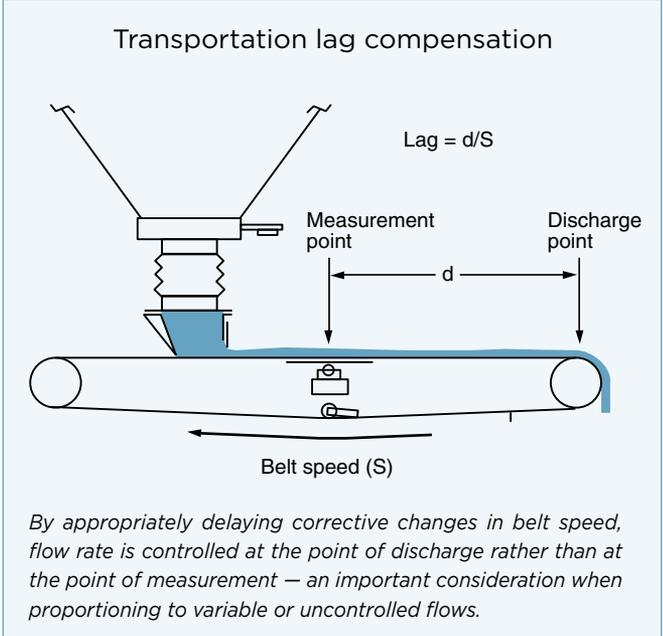
be applied in order as the corresponding belt segment passed over the weighing section.
