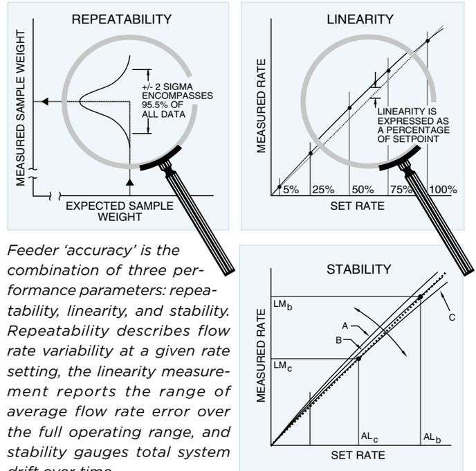
Feeder 'accuracy' is the combination of three performance parameters: repeatability, linearity, and stability. Repeatability describes flow rate variability at a given rate setting, the linearity measurement reports the range of average flow rate error over the full operating range, and stability gauges total system drift over time.
